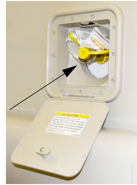
LP Accessory Connection (Located behind access door at the rear passenger side of the vehicle)
