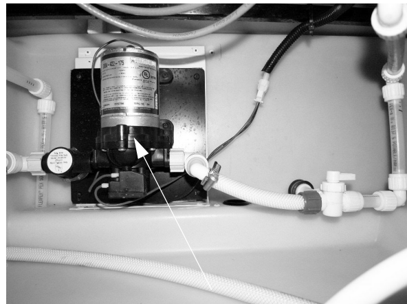
Water Pump -Typical installation shown (Located inside utility compartment (rear driver side compartment)).
