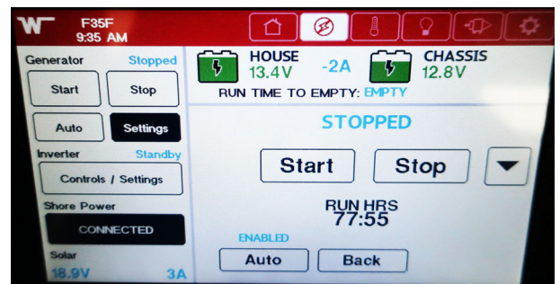
Generator Settings Screen Use this screen to customize various triggers to automatically start and stop the generator. Select the down arrow for further customizations and options. The total run hours are also displayed on this screen -Typical View
