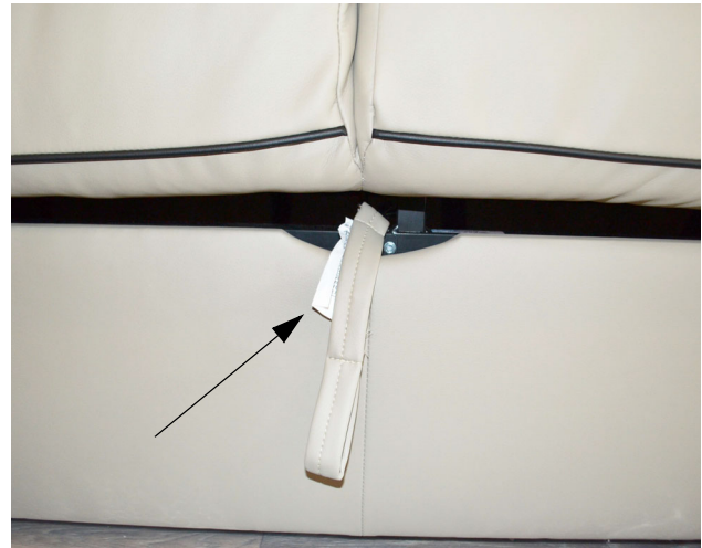
Security Latch Strap -Typical View
