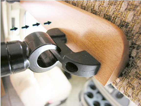
Attaching Bunk Ladder
